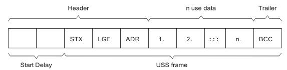
Figure 6-16 Structure of USS telegram
