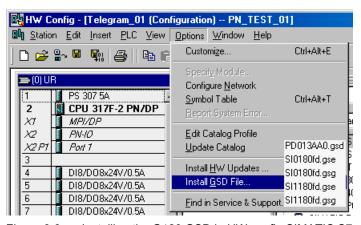
Figure 6-8 Installing the G120 GSD in HW config SIMATIC S7
