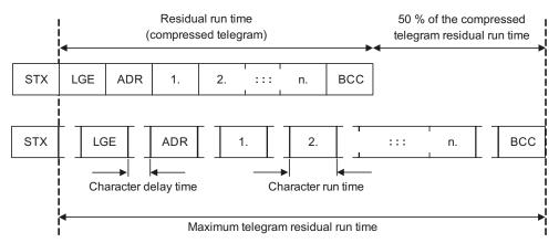
Figure 6-19 Residual Run Time and Character Delay Time
