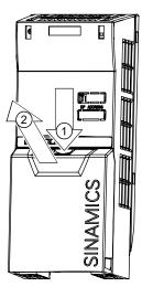
Figure 4-2 Removing the Control Unit terminal cover
