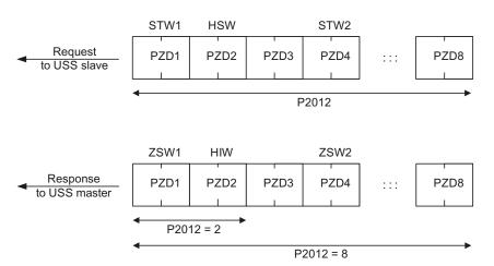
Figure 6-22 Process data channel
