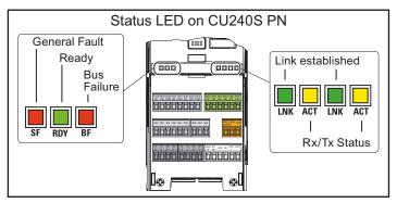
Figure 7-1 State LED on the CU240S, CU240S DP, CU240S DP-F, CU240S PN
