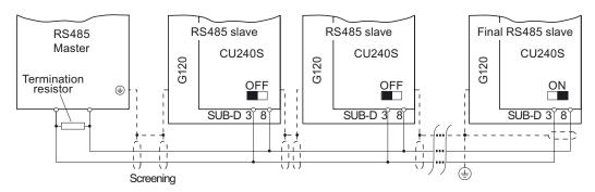
Figure 6-15 USS network via RS485
