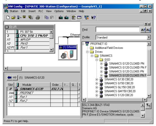
3. Double click onto e.g. "SINAMICS G120 CU240S PN F" to add the G120 inverter as I/O device to the subnet.
