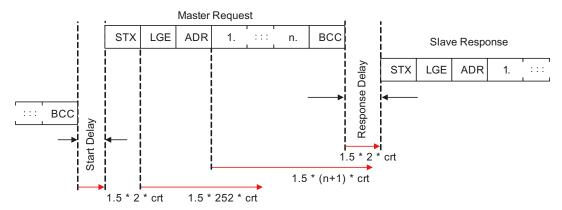
Figure 6-21 Timeout Checks on USS Slave
