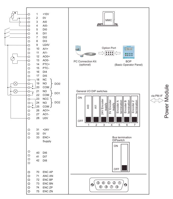
Figure 3-2 Block diagram CU240S
