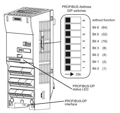
Figure 6-7 PROFIBUS DP address DIP-switches
