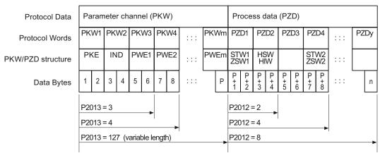
Figure 6-17 USS use data structure
