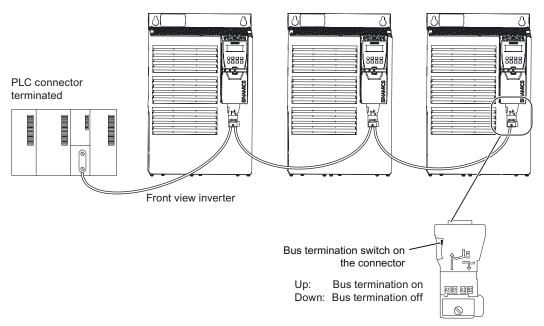
Figure 4-4 PROFIBUS network with bus termination
