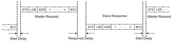
Figure 6-20 Start Delay and Response Delay
