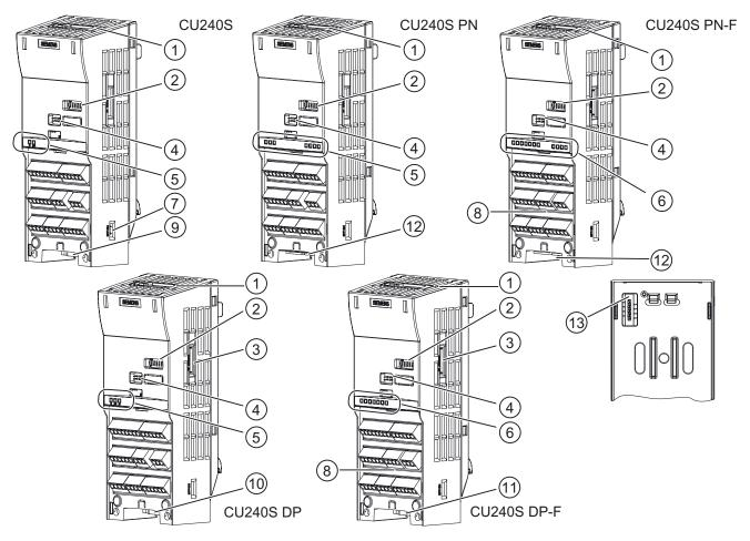
Figure 3-1 Control Units CU240S
