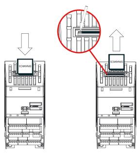
Figure 5-3 Fitting and Removing the MMC
