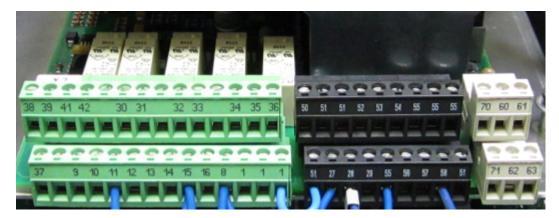
Figure 8-13 Control cable terminals
