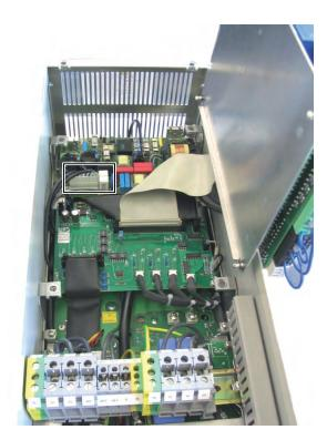
Compact device W=225, connector for external control voltage
