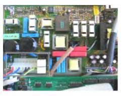
Switching power supply with connector on internal control voltage Switching power supply with connector on external control voltage
