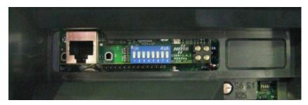
Figure 10-6 Modbus TCP board
