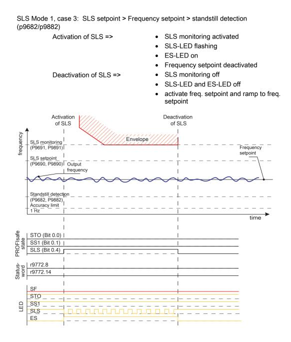
Figure 8-20 SLS Mode 1, case 3: SLS setpoint > Frequency setpoint > standstill detection (p9682/p9882)
