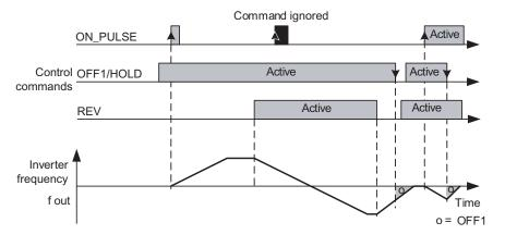
Figure 7-5 3-wire control using ON\_PULSE, OFF1/HOLD and REV
