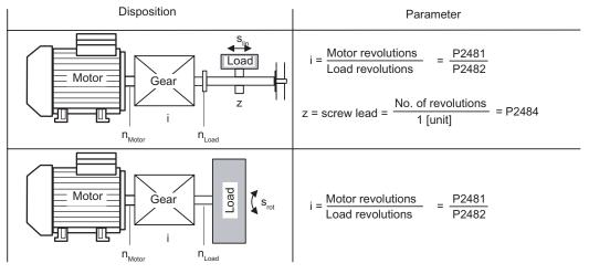
Figure 6-5 Rotary or linear axis
