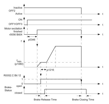
Figure 6-20 Motor holding brake after ON/OFF2
