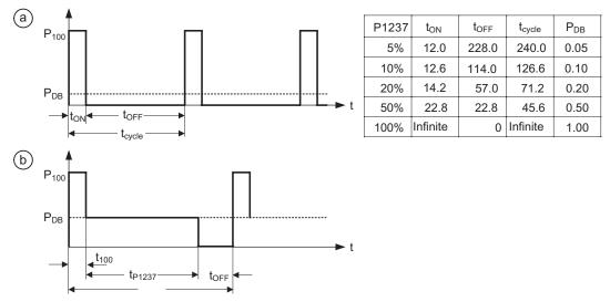
Figure 9-9 Chopper load duty cycle
