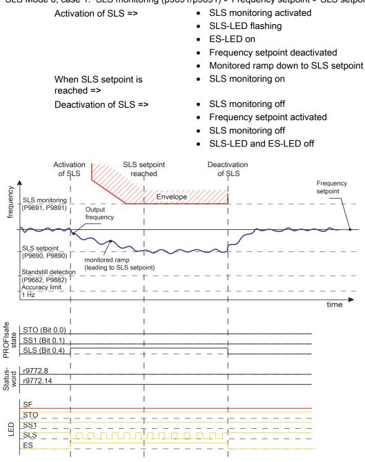
SLS Mode 0, case 1: SLS monitoring (p9691/p9891) > Frequency setpoint > SLS setpoint
