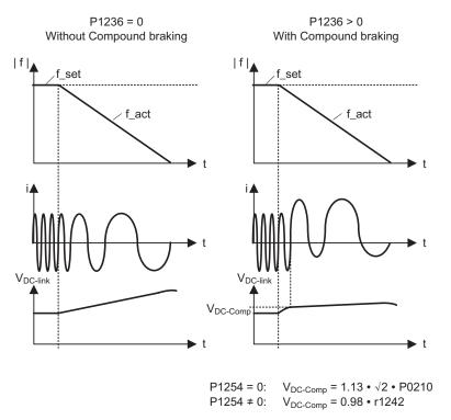
Figure 9-4 Compound braking
