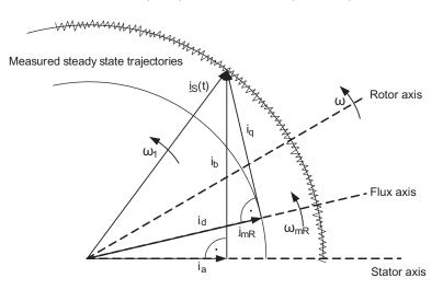
Figure 6-37 Current vector diagram in a steady-state condition
