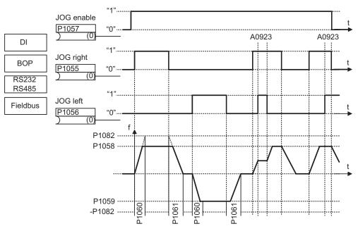
Figure 6-6 JOG counter-clockwise and JOG clockwise
