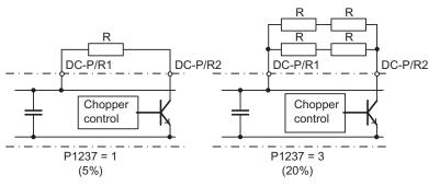
Figure 9-8 Increasing the level of braking energy which can be absorbed
