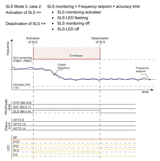
Figure 8-30 SLS Mode 3, case 2: SLS monitoring > Frequency setpoint > accuracy limit
