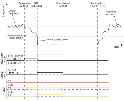
Figure 8-10 Safe Stop 1 (SS1) function
