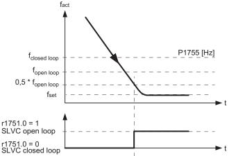
Figure 6-38 Changeover condition during ramp down for SLVC
