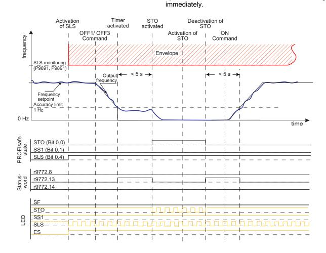
Figure 8-32 SLS Mode 3, case 4: Frequency setpoint drops below accuracy limit with user activation of STO
