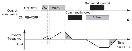
Figure 7-2 Siemens standard control using ON/OFF1 and ON\_REV/OFF1
