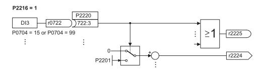
Figure 7-13 Directly selected PID fixed setpoint using DI3
