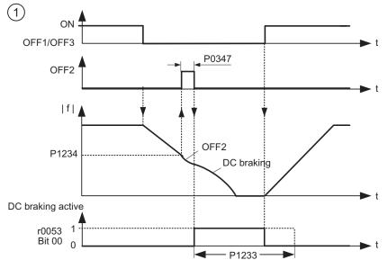
Figure 9-2 DC braking after OFF1/OFF3
