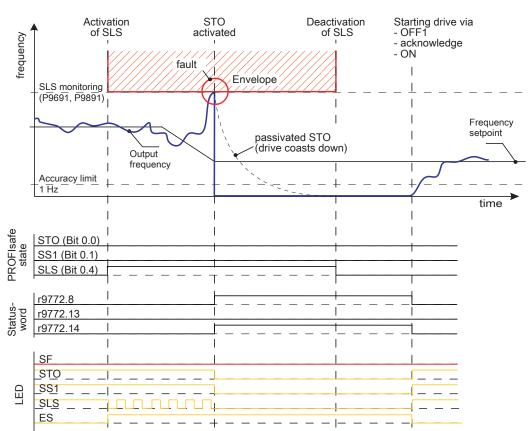
Figure 8-35 SLS Mode 3, case 7: SLS monitoring > Frequency setpoint
