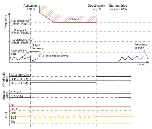
Figure 8-15 SLS Mode 0, case 4: accuracy limit > Frequency setpoint
