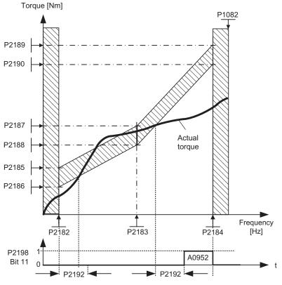
Figure 6-7 Load torque monitoring (P2181 = 1)
