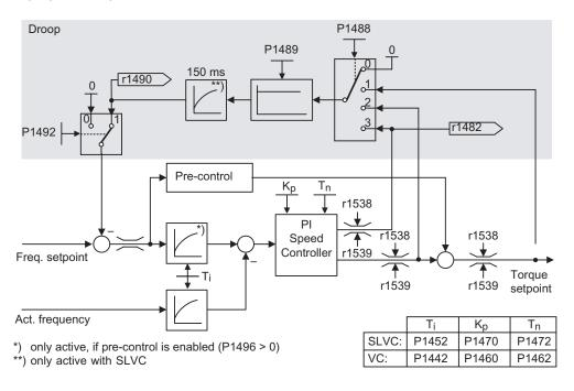
Figure 6-45 Speed controller with droop
