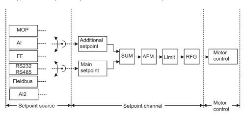
Figure 6-22 Setpoint channel
