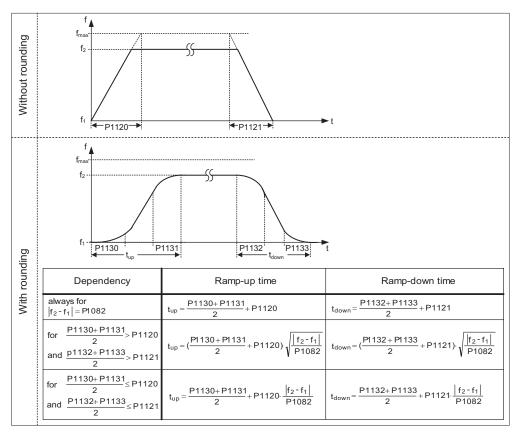
Figure 6-25 Ramp-function generator
