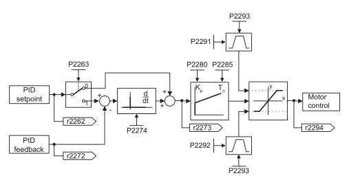
Figure 7-10 PID controller
