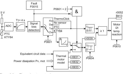
Figure 6-9 Thermal motor protection
