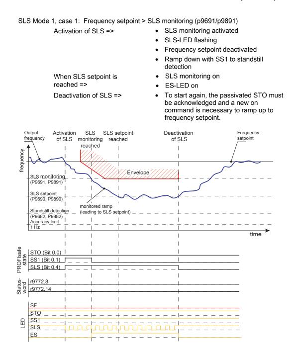
Figure 8-18 SLS Mode 1, case 1: Frequency setpoint > SLS monitoring (p9691/p9891)
