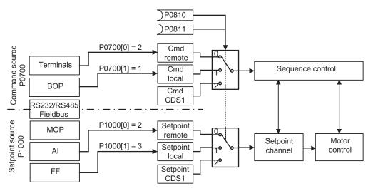
Figure 6-30 Changing-over using the BICO parameters P0810 and P0811
