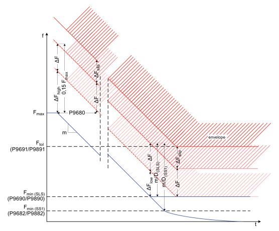
Figure 8-6 Safety limits for SLS and SS1
