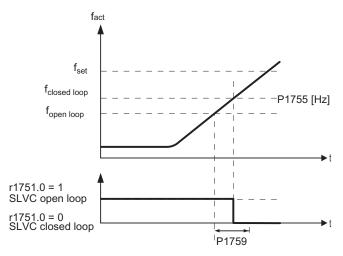
Figure 6-39 Changeover condition during ramp up for SLVC
