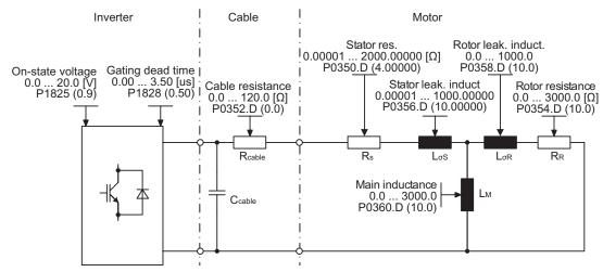
Figure 6-1 Equivalent circuit diagram (ECD)
