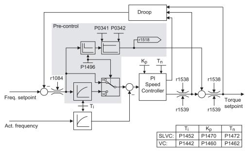
Figure 6-44 Speed controller with pre-control
