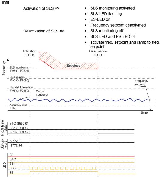
SLS Mode 1, case 4: Standstill detection (p9682/p9882) > Frequency setpoint > accuracy
