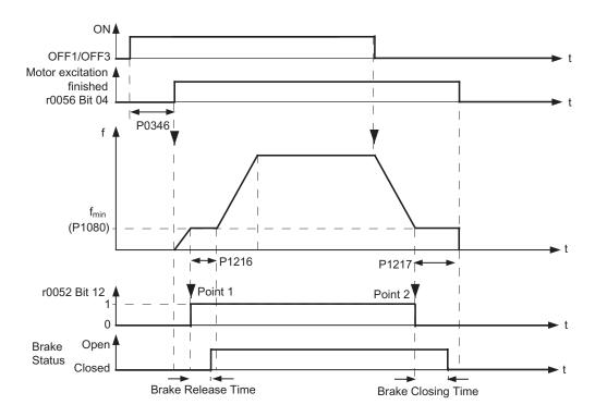
Figure 6-19 P1215 Motor Holding Brake OFF1/Off3
