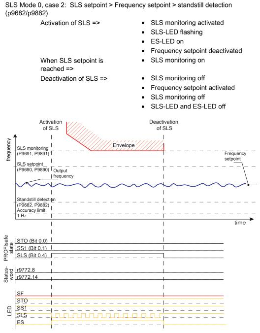
Figure 8-12 SLS Mode 0, case 2: SLS setpoint > Frequency setpoint > standstill detection (p9682/p9882)
