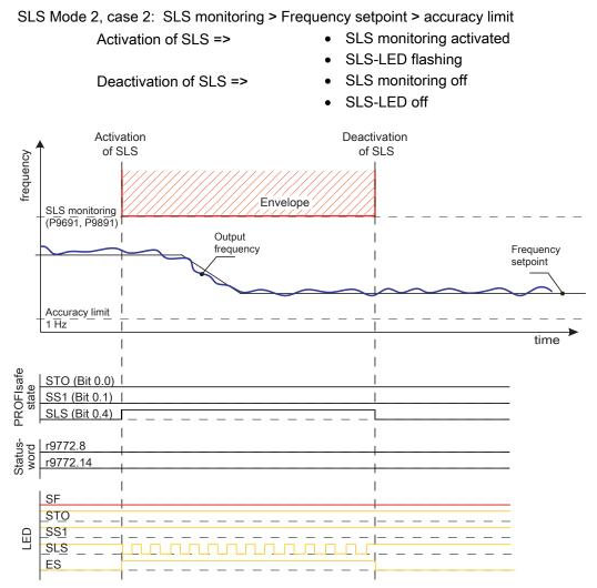
Figure 8-26 SLS Mode 2, case 2: SLS monitoring > Frequency setpoint > accuracy limit
