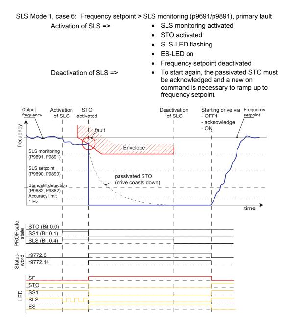
Figure 8-23 SLS Mode 1, case 6: Frequency setpoint > SLS monitoring (p9691/p9891), primary fault
