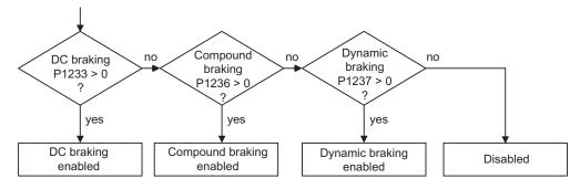
Figure 9-1 Inter-dependency of electronic brakes
