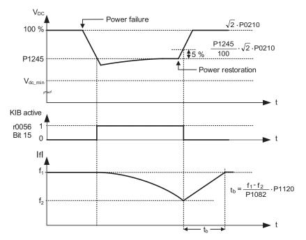
Figure 9-12 Kinetic buffering (Vdc\_min controller)
