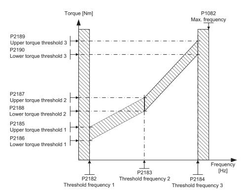
Figure 6-8 Frequency and torque tolerance bandwidth
