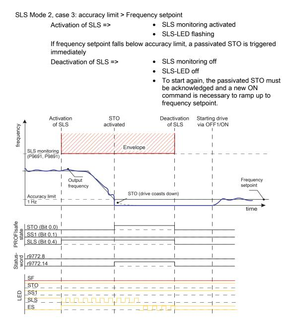
Figure 8-27 SLS Mode 2, case 3: accuracy limit > Frequency setpoint
