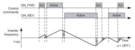
Figure 7-3 2-wire control using ON\_FWD and ON\_REV
