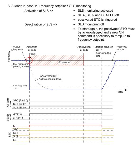
Figure 8-25 SLS Mode 2, case 1: Frequency setpoint > SLS monitoring
