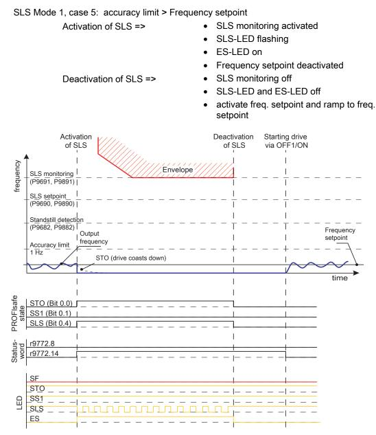
Figure 8-22 SLS Mode 1, case 5: accuracy limit > Frequency setpoint
