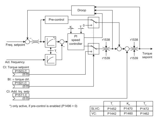
Figure 6-46 Closed-loop speed and torque control
