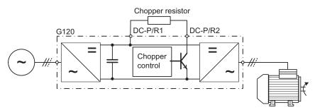
Figure 9-5 Connecting the chopper (braking) resistor
