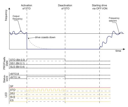
Figure 8-8 Safe Torque Off function
