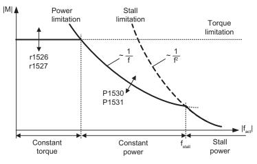
Figure 6-48 Torque limits
