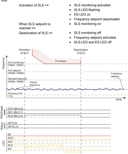
SLS Mode 0, case 3: Standstill detection (p9682/p9882) > Frequency setpoint > accuracy limit
