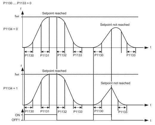
Figure 6-26 Rounding-off after an OFF1 command
