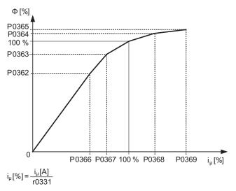
Figure 6-2 Magnetizing characteristic
