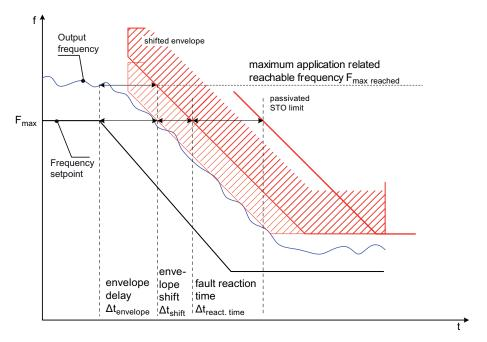
Figure 8-7 Maximum fault reaction time
