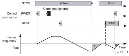
Figure 7-4 3-wire control using FWDP, REVP and STOP
