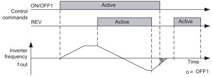
Figure 7-1 Siemens standard control using ON/OFF1 and REV
