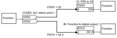
Figure 5-3 Connector output/Binector output (CO/BO)
