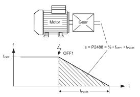
Figure 6-4 Positioning ramp down
