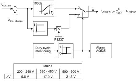
Figure 9-6 Mode of operation of the dynamic braking
