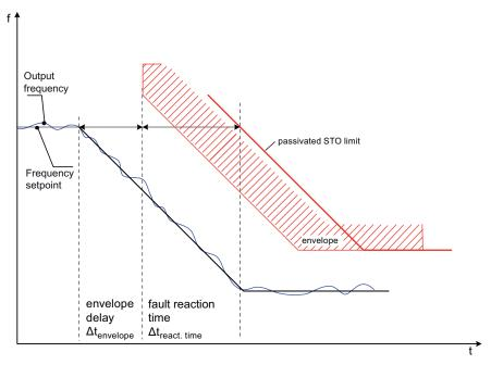
Figure 8-5 Maximum shut-down time
