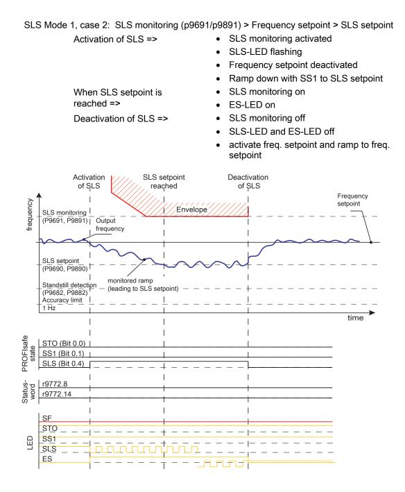
Figure 8-19 SLS Mode 1, case 2: SLS monitoring (p9691/p9891) > Frequency setpoint > SLS setpoint
