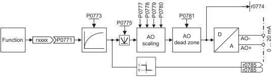
Figure 7-18 D/A converter channel
