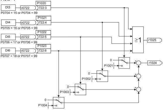
Figure 7-6 Direct selection of fixed frequencies - functional overview
