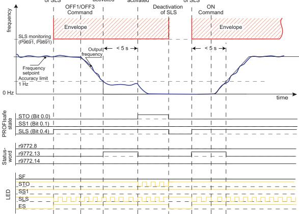
Figure 8-31 SLS Mode 3, case 3: Frequency setpoint drops below accuracy limit after activation of SLS
